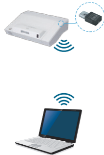
Without an access point
